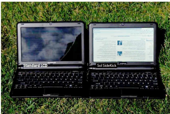
Reflective mode outdoors - Sol SideKick backlight turned off. Standard LCD can not operate at high ambient light levels.
